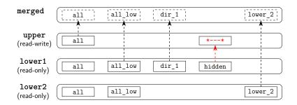
• Read-write upper layer is "diff" applied to lower layers
